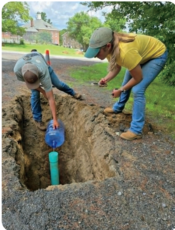
← Suozzo, Doty & Associates field staff check for soil types, and infiltration falling-head permeability. These tests will determine what types of green infrastructure will work best for the project site.
